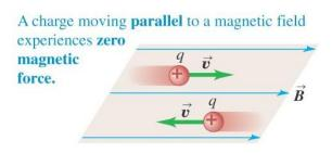
A charge moving at an angle  $\phi$  to a magnetic field experiences a magnetic force with magnitude  $F = |q|v_{\perp}B = |q|vB \sin \phi$ .
