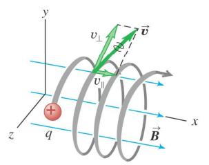
A charged particle will move in a plane perpendicular to the magnetic field.
