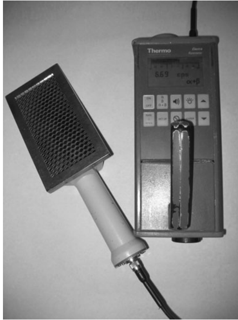
Figure 9.7 Dual ( \alpha and \beta ) contamination probe and ratemeter.
